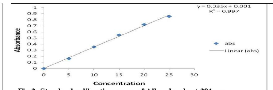
Fig.2: Standard calibration curve of Albendazole at 291 nm.
