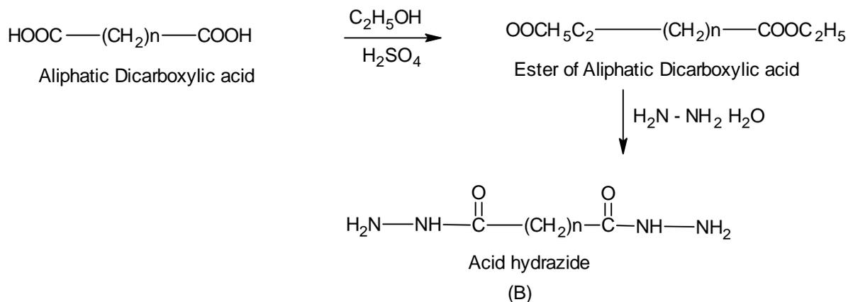
The acid (0.1 mole) and absolute ethanol (50 ml) were taken with a few drops conc. H<sub>2</sub>SO<sub>4</sub> and was refluxed for 6 hours. The reaction mixture was concentrated by distilling off the excess of ethanol under reduced pressure. The ester obtained was used for the preparation of hydrazide directly.
