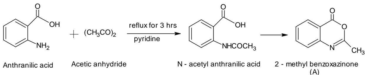
A Mixture of anthranilic acid (0.12 mol) in acetic anhydride (0.2 mol) with few drops of pyridine was refluxed for 3hr. The reaction mixture was filtered, washed and recrystallised from absolute ethanol, to get the crystals of 2-methyl 1,3,4- benzoxazinone(A). The physical data of compound (A) are summarized in **Table-1**.
