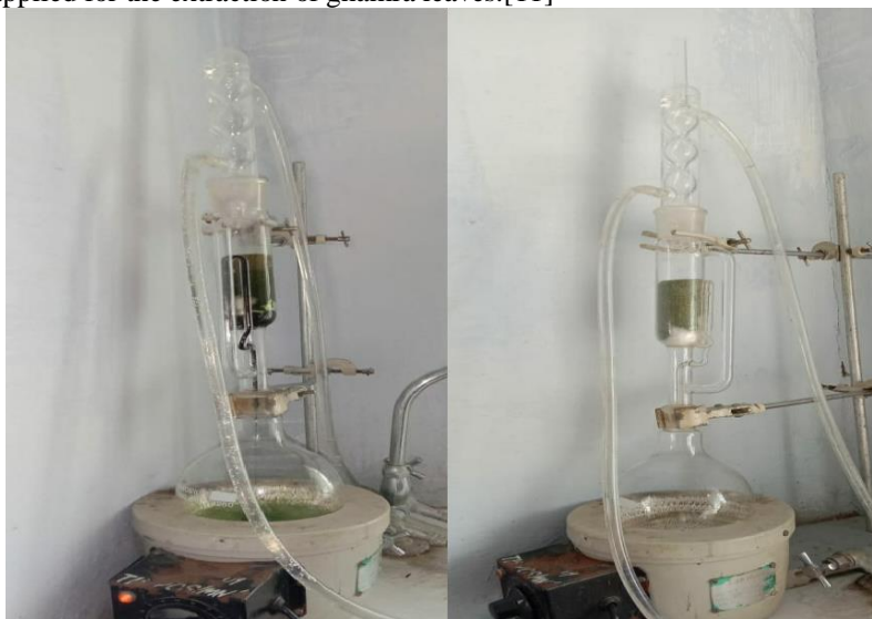
Figure 2: Extraction procedure for ghamra & neem.
