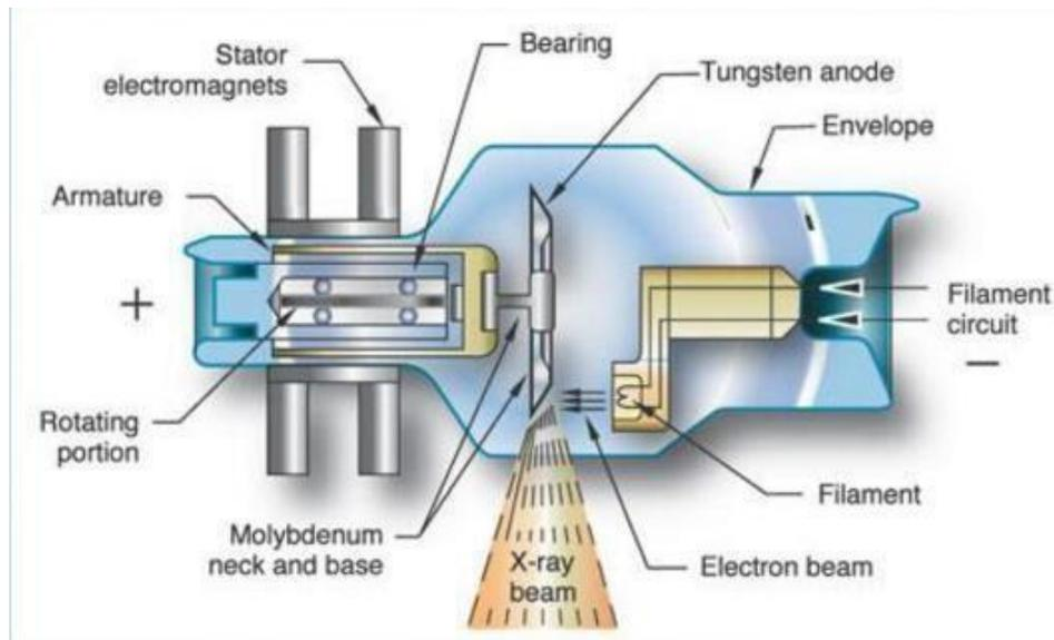
Figure 5. X-ray tube elements
