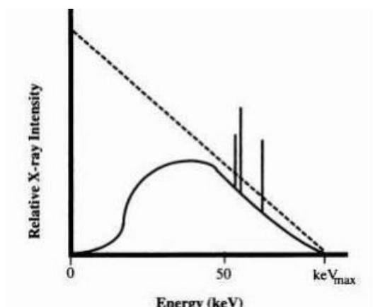
**Figure 3. Spectrum of emission to a tungsten target.**
