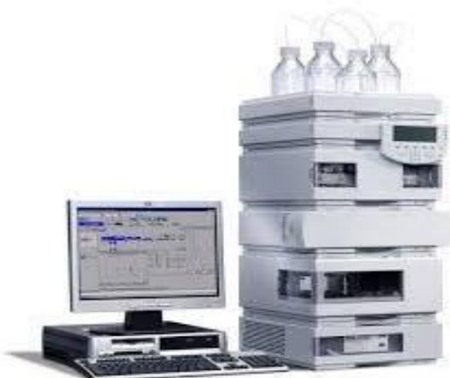
Fig no1: High Performance Liquid Chromatography
