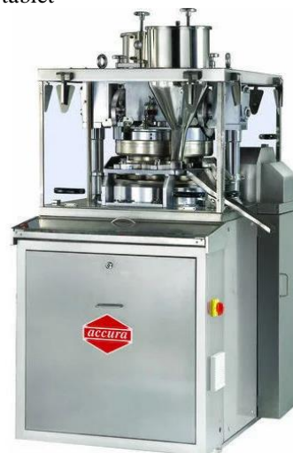
Fig 5: Single sided tablet press
