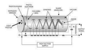
PMT can detect very weak signals, even 200 times weaker than that could be done using photovoltaic cell. Hence it is useful in fluorescence measurements. PMT should be shielded from stray light in order to have accurate results.
