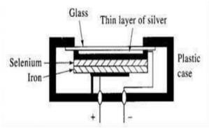
The detector has a thin metallic layer coated with silver or gold and acts as an electrode. It also has a metal base plate which acts as another electrode. These two layers are separated by a semiconductor layer of selenium. Selenium has extremely low electrical conductivity and hence the electrons are not mobile.
