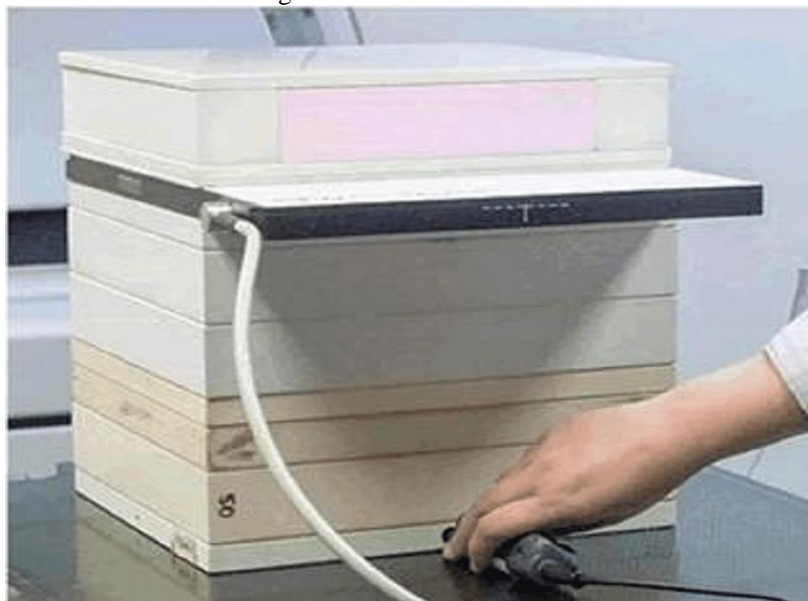
Figure 1: The initial evaluation setup utilizing an ionization chamber.
