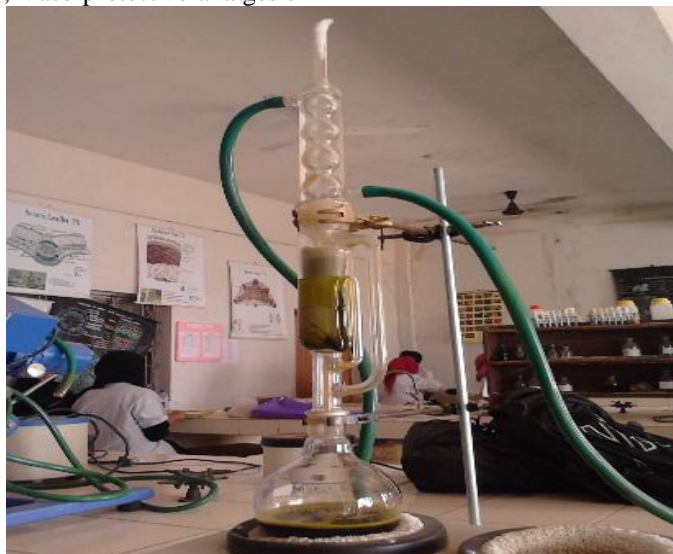
Figure 01: Extraction by soxhlet extraction technique.
