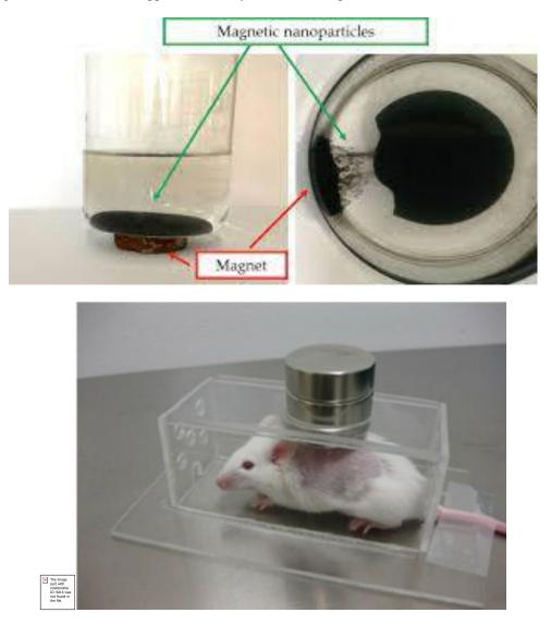
The following picture depicts the bio-distribution of magnetic nanoparticles after administration into the body. When administered intravenously the particles travel to the required site and concentrate at the site of action under the influence of the magnetic field provided by the external magnet assembly placed outside the body[14]
