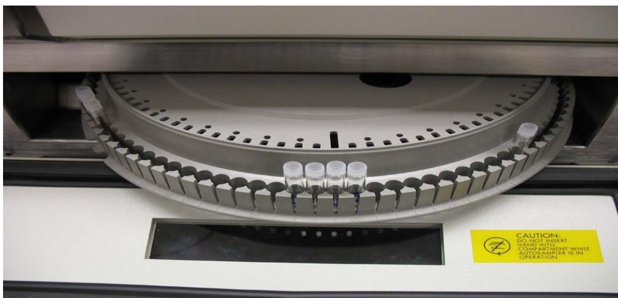
Inside of an autosampler for running several samples without user interaction, e.g. overnight [ fig-2]
