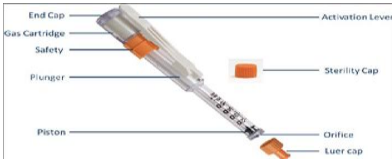
Figure 2. Schematic representation of injection via typical Needle-free system
