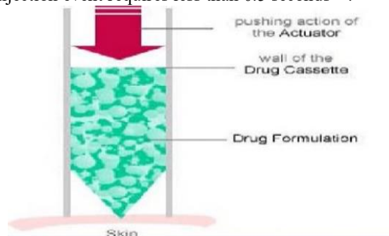
Figure 6. Mechanism of working of needle free injection system
