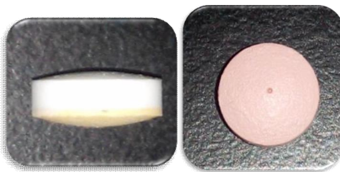
Figure 1: Upper and side view of coated osmotic tablet by drilling
