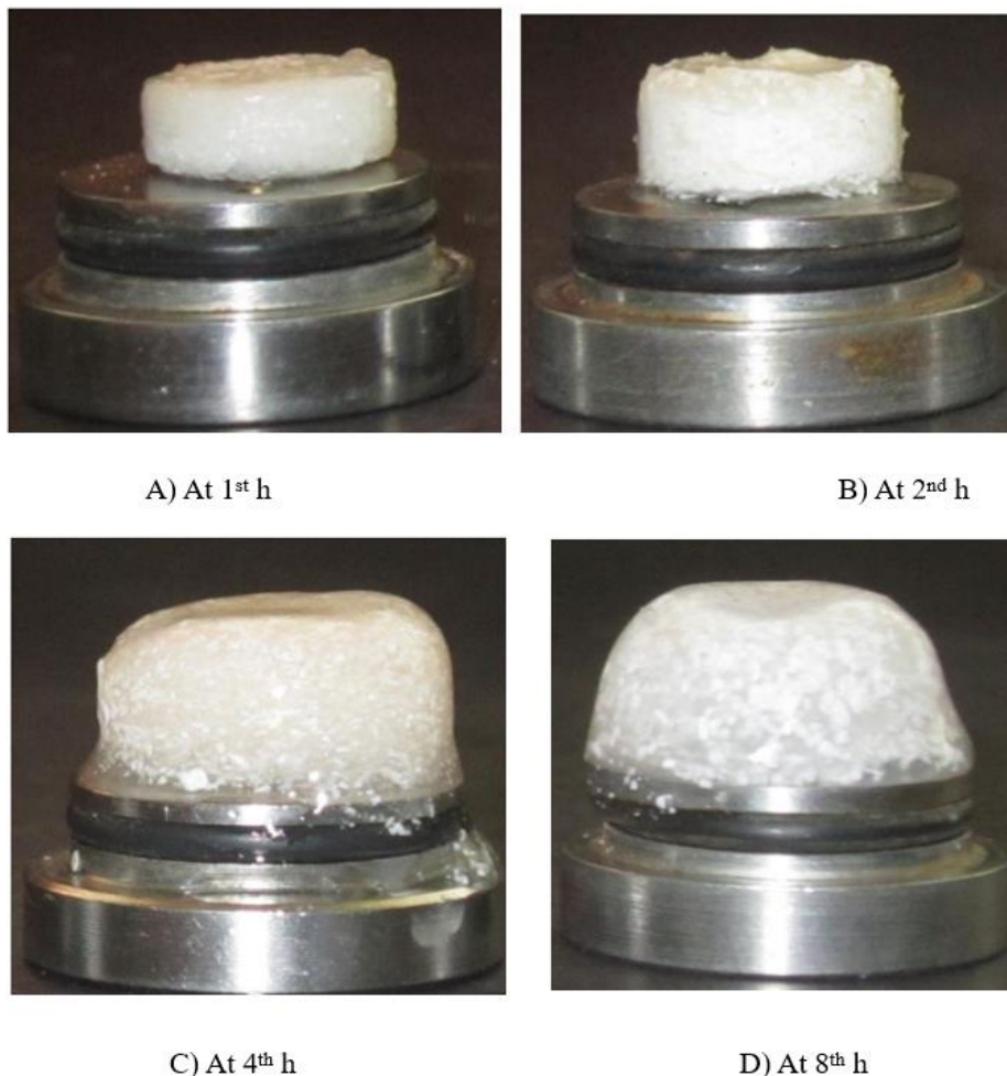
Figure 7: The floating matrix tablet formulation swells in a pH 1.2 HCl buffer, as shown in the photographs
