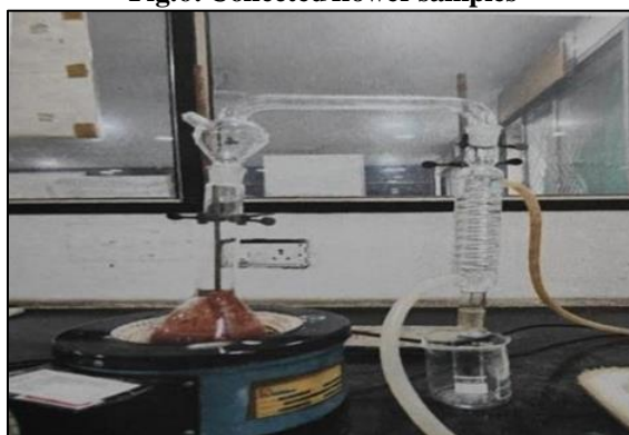
Fig.7: Extraction of hibiscus oil by steam distillation
