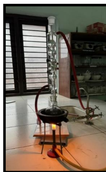
Fig.11. Saponification Value Determination
