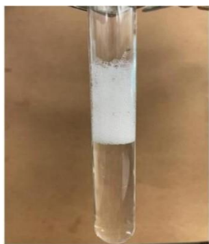
Figure 8 Froth Test for Detection of Saponin.
