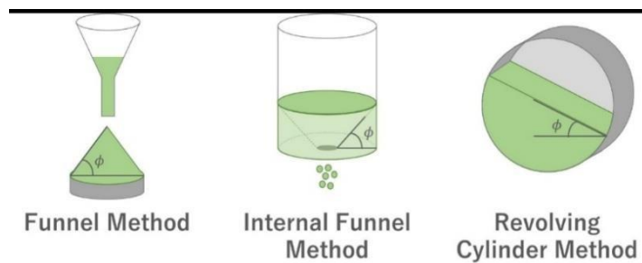
Figure 7 Flow Property Evaluation of polyherbal powder
