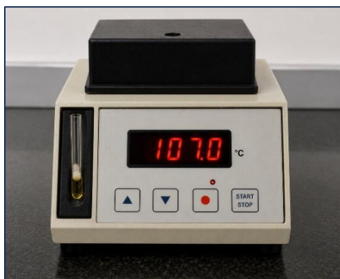
Fig. 3: Melting Point Determination of Pentoxifylline Using Capillary Method
