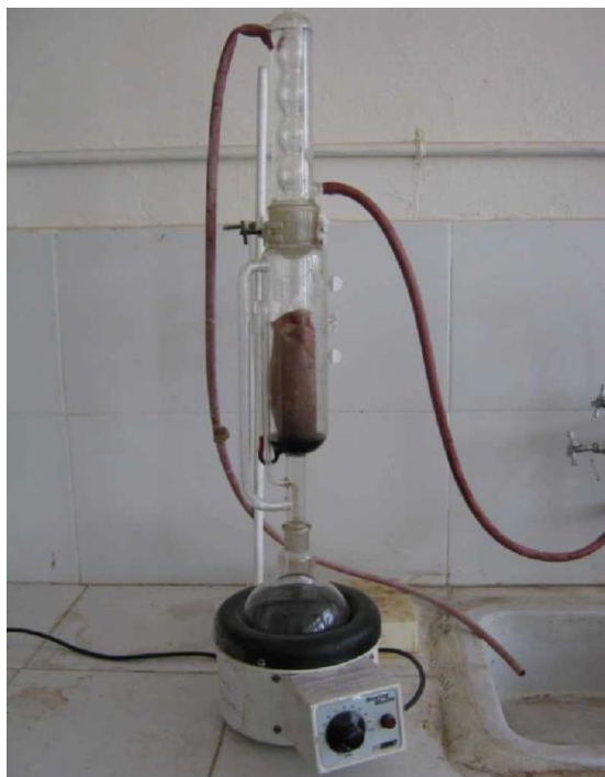
Figure 7.1 Soxhlet apparatus for the extraction of different plant Extracts
