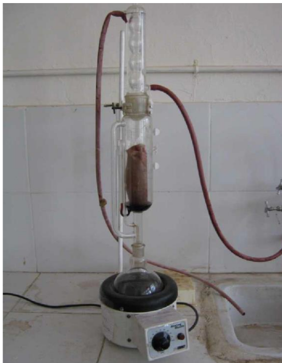
Figure 4.5 Soxhlet apparatus for the extraction of different plant Extracts
