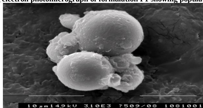
Figure 2: Scanning electron photomicrograph of formulation F2 showing population of microspheres
